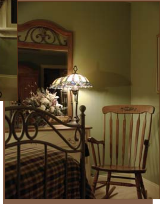
(Figure 1) Conceal light source within opaque shade (left) or diffuse glass (below) to protect eyes from glare.
